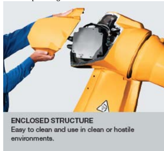
Fig. 4 - STAUBLI TX 200 Robot. This picture is the property of STAUBLI [2]
